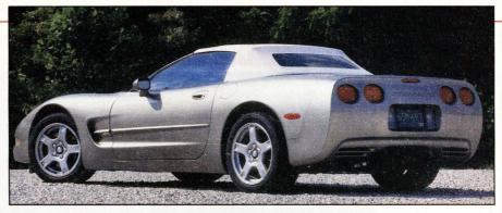
Designed from the outset as a convertible with a rigid chassis, the Corvette has an easily used manual folding roof, a hard tonneau with molded vestigial head fairings, and what Chevy calls a "waterfall" between the seats (below) that evokes the original 1953 model.
